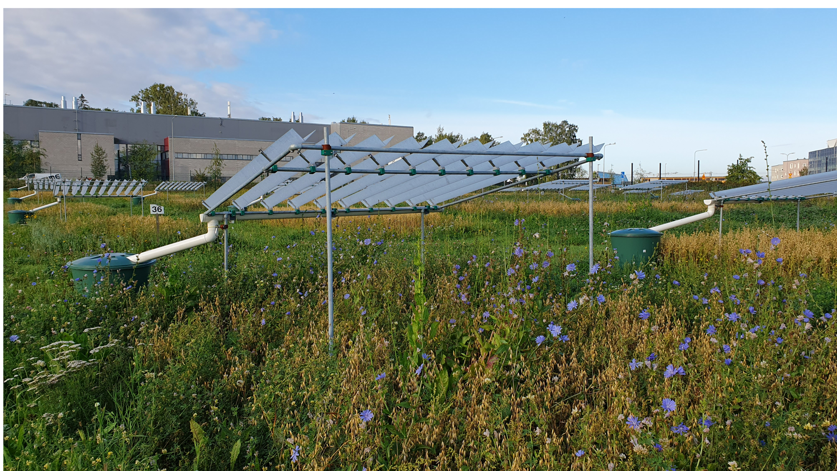
Figure 2. Rainout shelters (Kundel et al. 2018) installed as a split-plot design. Photo by Pauliina Turunen.
